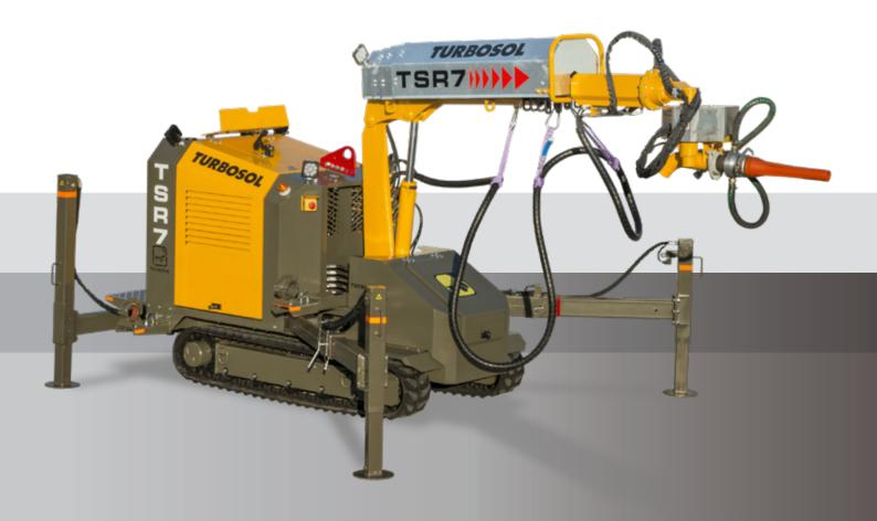
TSR 7: crawler equipment designed for shotcrete applications in jobsites with difficult access and tunnels.
