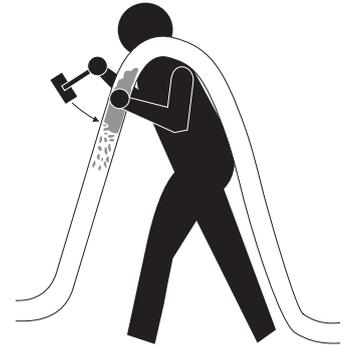
Start the pump for a few moments and ensure that the hose is free of the plug: the material should flow out freely.
