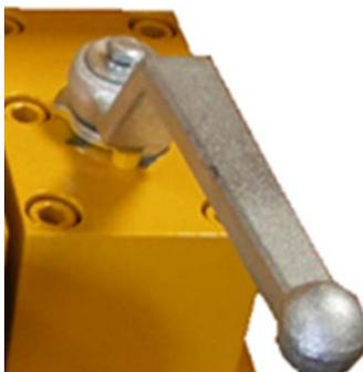
S-TUBE SHIFT SELECTOR BALL VALVE controls the speed of the S-Tube shift.
