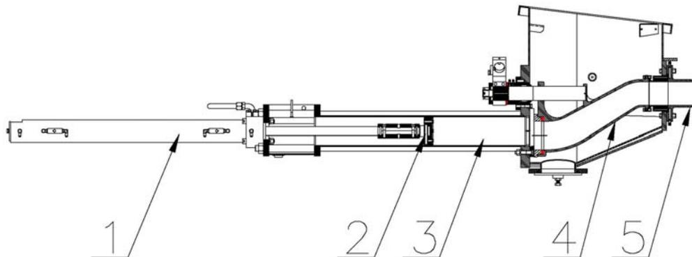
The hydraulic oil flow created by the hydraulic pump pushes the drive cylinder pistons inside the drive cylinders (1) alternately back and forth. Because the drive cylinders and concrete pistons (2) inside the concrete cylinders (3) are linked together, the pistons move synchronously.
