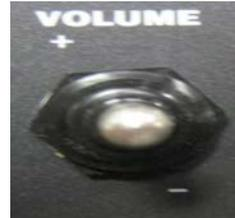
VOLUME CONTROL KNOB or SWITCH adjusts volume output of the material
