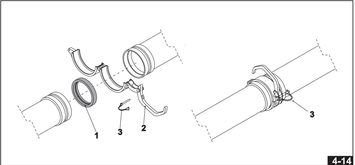
Connect the mortar conveyor piping 1 (Fig. 4-15).
