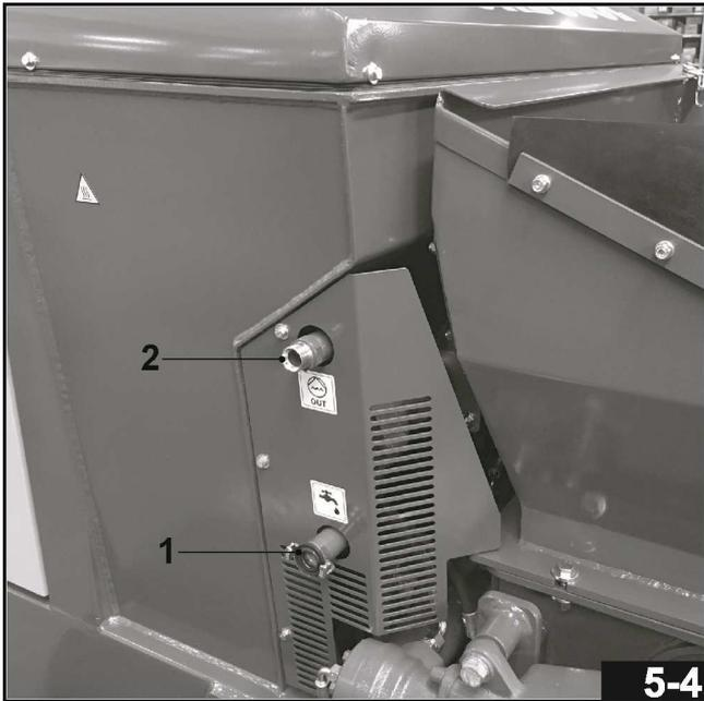
Connect the water intake pipe to the supply fitting 1 (FIG.5-4).
