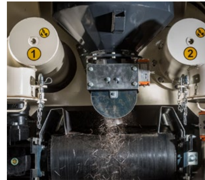
Metal fibres dispenser - dosing by weight
