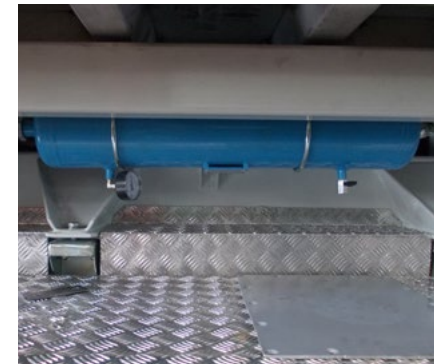
Air cannon in the sand compartment
