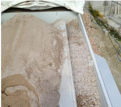
Mobile adjustable bulkhead for the sand compartment
