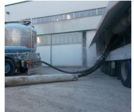
Pneumatic refilling system for cement compartment
