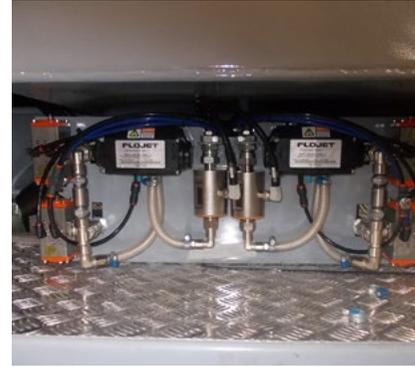
Flow sensor for liquid additives dosing
